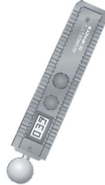
Equipment for structural moisture analysis (V1-D4 Pro)
